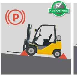
This important safety system is activated when the engine stops, when the Operator Presence Safety System (OPSS) detects a fault, or the transmission is placed in neutral. If the operator needs to use the parking brake while the engine is running, it can be quickly applied and released with just the touch of a dedicated button.
