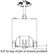
12.4" to top of pin in highest position 4.5" powered lift range
