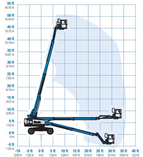
(1) The metric equivalent of working height adds 2 m to platform height. The imperial equivalent adds 6 ft to platform height.
