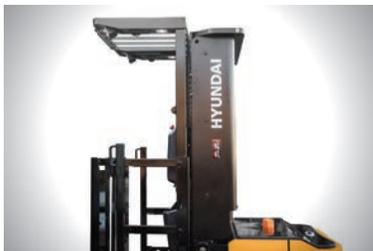
**Mast cover : Platform control system protection**
