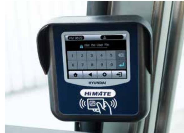
Hyundai Hi-Mate is our exclusive remote management system available for the LC-9 Series and other Hyundai forklifts. This innovative system uses cellular technology to provide real-time data 24/7. The richness of the data and the communication and control it provides can transform your workplace.
