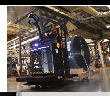
The Big Joe AMR features an easy to learn user interface accessed via the onboard touchscreen, allowing you to set-up, map and start missions in less than one hour. If you can use a smartphone, you can program the Big Joe AMR!
